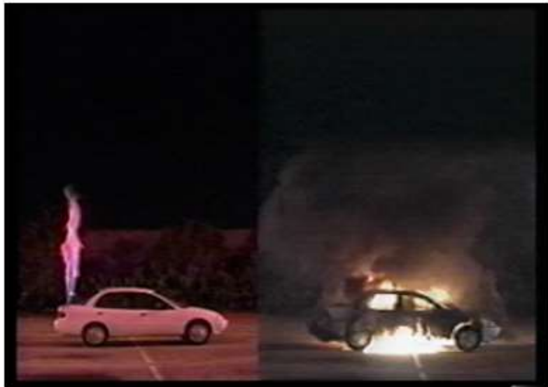
Photo 3 - Time: 1 min, 0 sec - Hydrogen flow is subsiding, view of gasoline vehicle begins to enlarge
